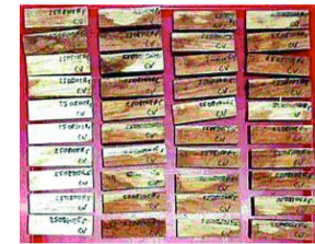
Standardised test samples coming from various parts of oak after exposure to Corioliolus versicolor during 16 weeks.
